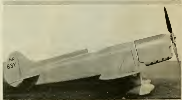
The Brown Special, powered with the 4-cylinder 185-h.p. Menasco C-4-S Pirate engine
